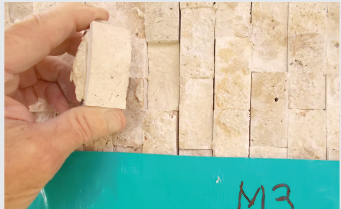
Merkrete's Pro Epoxy's bond proved stronger than the travertine – the stone sheared in two.
