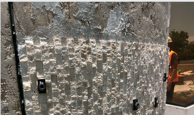
Pull tests ensured Merkrete's Pro Epoxy had the required tensile strength for the job.
